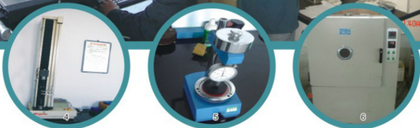
1、Oil seal rotary performance testing machine 2、Auto shock absorber testing machine 3、Motorcycle shock absorber testing machine 4、Tensile Machine 5、Durometer 6、Ageing Oven 7、Projector 8、Lab
